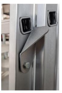
The segment hooks are used to adjust ladder height step by step. The segment lock is used to lock the ladder at the desired height, so that the ladder can be moved and lifted.
