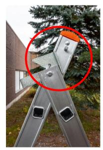
Limiter strap is loose. Do not climb onto the ladder!
